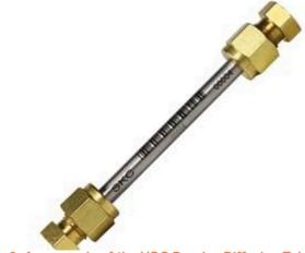
Photo 3: An example of the VOC Passive Diffusion Tube used in the study.
