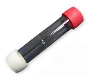
Photo 4: An example of the Passive Diffusion Tube used to monitor  $SO_2$ ,  $O_3$  and  $NO_2$  in the study.
