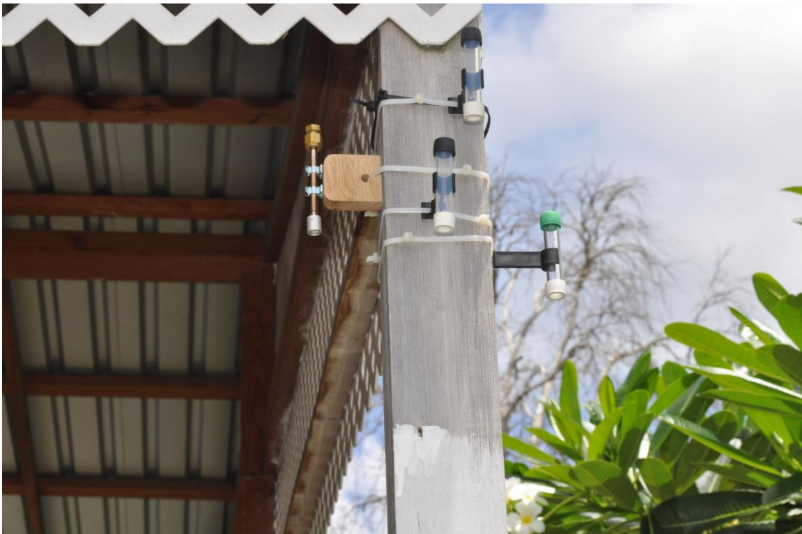
Photo 4: Passive samplers mounted at Pickwick Gap, St. Michael
